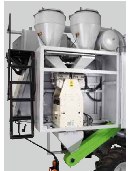
The 2 pre-containers are opened and the harvested material falls into the weigh bucket
