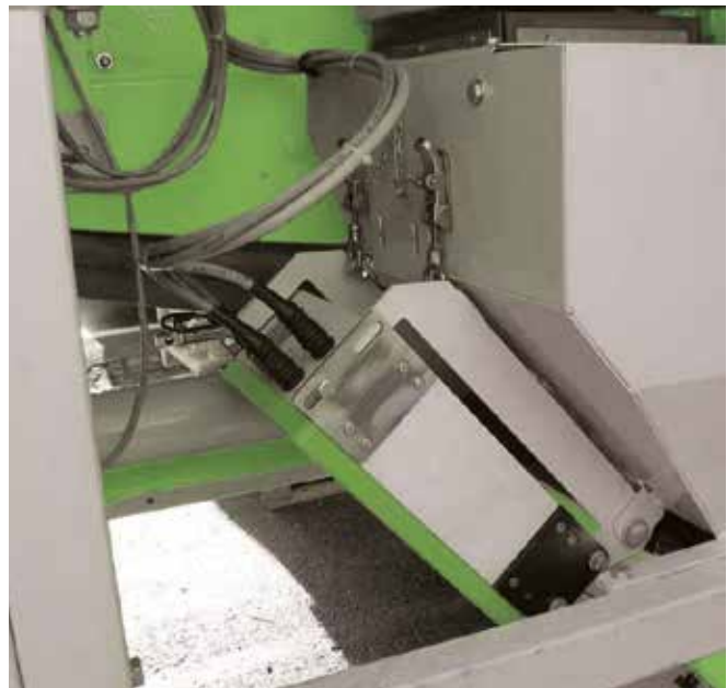
NIRS measuring installed on the weighing system
